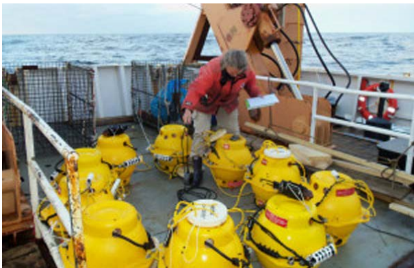
Marine autonomous recording units, or MARUs, fill the deck before deployment in the sanctuary. Credit: NOAA/NEFSC.
