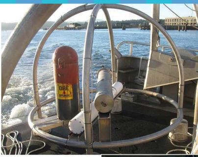
An Autonomous Underwater Hydrophone (AUH) package was deployed in the sanctuary. The echosounder image at right shows the equipment as it was lowered 200 feet down to the seafloor. The station is located in the proposed Designated Habitat Research Area-Northern Reference Area. Credit: SBNMS.
