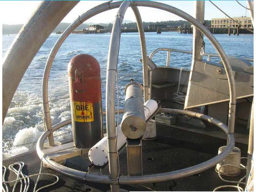
An Autonomous Underwater Hydrophone (AUH) package was deployed in the sanctuary. The echosounder image at right shows the equipment as it was lowered 200 feet down to the seafloor. The station is located in the proposed Designated Habitat Research Area-Northern Reference Area. Credit: SBNMS.
