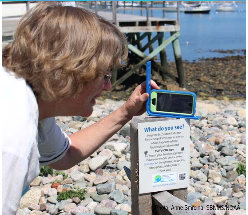
A smartphone owner takes a photo of Scituate Harbor using the ICUC bracket. All photos from this station will record the same landscape with any changes over time.
